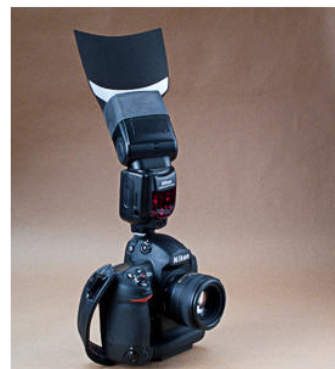
ABBC PRO bouncing around the room Black Foam Cut To Size - White Reflector Tape Applied
